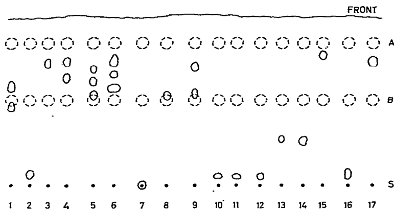
Fig. 3. One-dimensional chromatographic separation of dansyl-cyclic-3',5'-AMP and metabolites on a silica gel thin-layer plate (15 × 15 cm). The solvent system used was n -butanol saturated with 0.1 N HCl. A = dansyl-NH 2 ; B = dansyl-OH. S = starting point; 1 = dansyl-xanthosine; 2 = dansyl-ADP; 3 = dansyl-guanine; 4 = dansyl-guanosine; 5 = dansyl-adenosine; 6 = dansyl-inosine; 7 = dansyl-ATP; 8 = dansyl-cytidine; 9 = dansyl-hypoxanthine; 10 = dansyl-2'-AMP; 11 = dansyl-3'-AMP; 12 = dansyl-IMP; 13 = dansyl-cyclic-2',3'-AMP; 14 = dansyl-3',5'-AMP; 15 = dansyl-cytosine; 16 = dansyl-AMP; 17 = dansyl-adenine. Note: more than one dansyl derivative is formed for compounds 1, 4, 5, 6 and 9.
